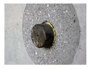
Bond the test dolly to the test area
