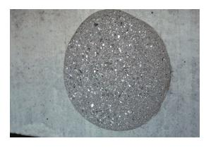
The prepared test locations must have a diameter between 10 and 20 cm
