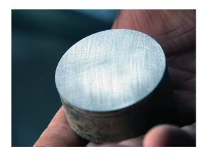
Roughen the test dolly crosswise with sandpaper, then clean with S&P Cleaner and de-grease
