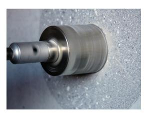
Check of the dew point and substrate moisture content by S&P
