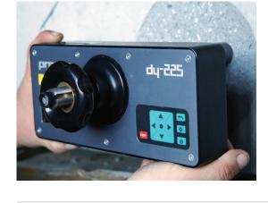
Fix the test machine carefully onto the bolt
