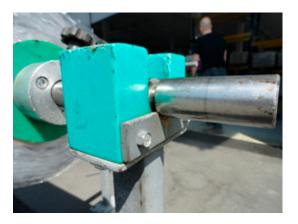
Put the rod on the support by aligning the rod's grooves with the plates on the supports and slotting them in place.
