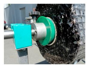
Align the S&P asphalt reinforcement with the roller below it using the adjustable taper.
