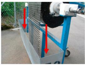
The S&P asphalt reinforcement must unroll within the plate guard.
