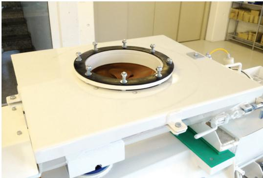
For silo: Attach using the pre-installed connectors on the silo (no dust development)
