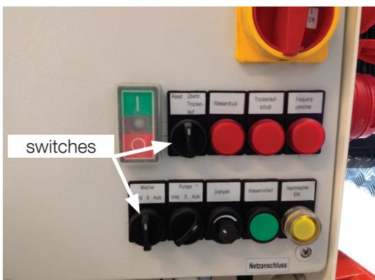
Before the end of the spraying work, set the «Mischer» (Mixer) rotary switch to «O» and set the rotary switch to «Überbr. Trockenlauf» (bypass dry run) to pump the remaining material out of the post-mixing container until the delivery shaft can be seen.
