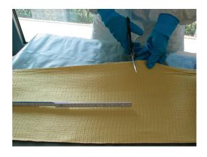
Tailor the S&P A-Sheet 120 to size using industrial scissors.
