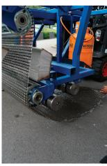
Regularly spray the rollers and tyres during installation with a separating agent.
