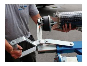
Open the clamp, attach the roll and secure the clamp again.
