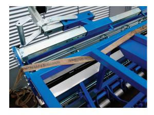
Remove the unloading belts and unscrew the 4 securing screws.
