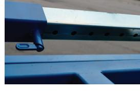
Adjust the roll bar to the desired width and secure with the latches
