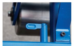
Open the safety latch and remove the support legs.
