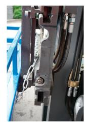
Feed the safety chain behind the forks and secure it.
