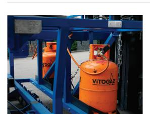
Correctly position the gas canisters, attach the tubes and secure with the safety chain.
