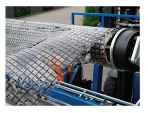
Pull approximately the first 3 metres of the roll manually, then bend it back and feed it over the upper roller.
