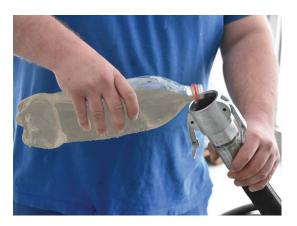
Before starting the material conveying, a lubricating mixture must be added to the material hoses! This can be a cement slurry, but we recommend using fish paste.
