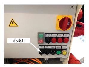
Set the «Mischer» (mixer) rotary switch to «Auto» and wait until the entire post-mixing container is full. The mixer stops automatically as soon as the mortar reaches the probe.
