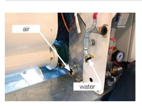
Connect the compressed air and the water to the S&P ARMO-Power Pump. Air and water pressure maximum 2 bar (29 psi).
