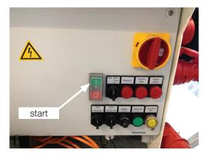
When the indicator light goes off, the green system power button can be pushed to start the pump.
