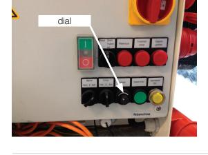
Turn the pump speed dial «Drehzahl» to the desired position. This can be used to set the delivery rate of the mortar.
