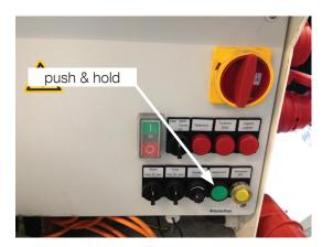
Push and hold the button «Wasservorlauf» (water supply) and adjust the waterflow with the handwheel.
