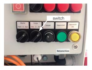
Set the rotary switch «Pumpe» to «Auto». Now the machine can be switched on and off at the spray nozzle. Air open: Machine starts pumping, air closed: Machine stops pumping.
