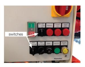
Before the end of the spraying work, set the «Mischer» (Mixer) rotary switch to «O» and set the rotary switch to «Überbr. Trockenlauf» (bypass dry run) to pump the remaining material out of the post-mixing container until the delivery shaft can be seen.
