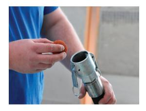
Now the machine and the material hoses can be cleaned. Each hose is to be cleaned individually and must be cleaned through at least 2 times with the cleaning balls.
