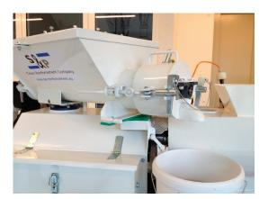
Turn the mixer to the side and let out at least one bucket of mortar until the material has a constant, homogeneous consistency. The mortar can be corrected to the desired amount of water using the handwheel. Then position the mixing unit again over the remixing container.
