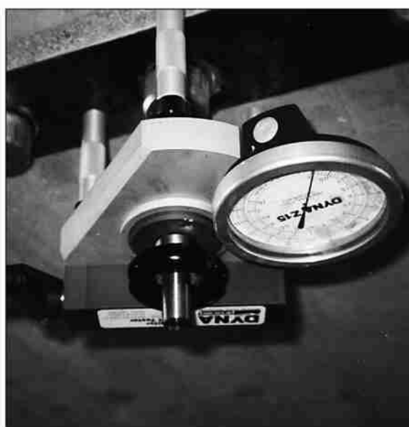
Fig. 3: Proceq Dyna Pull-off Tester used for determining substrate tensile strength
