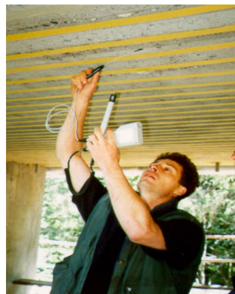
Fig. 7: Checking of substrate humidity
