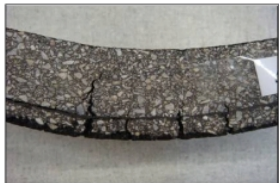
Image 3: Sample with S&P Carbophalt G 200 kN as interlayer
